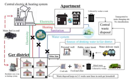
Figure 6. Lack of infrastructure in ger area of Ulaanbaatar city.
