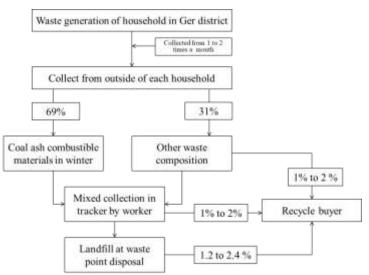
**Figure 8.** The proceeding of current dispose of municipal waste of ger district in Ulaanbaatar [8][10].
